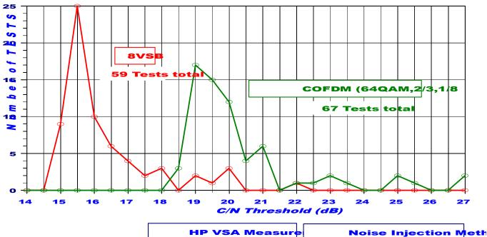
Statistics: 8VSB: Median = 15.7 dB Average = 16.4 dB Minimum = 15 dB COFDM: Median = 19.6 dB Average = 20.3 dB Minimum = 18.7 dB
