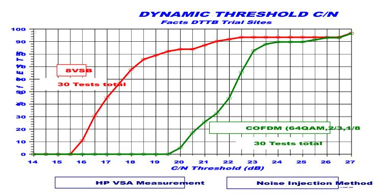
The distributions provide an indication of the spreads involved in C/N thresholds with particular differences between 8VSB and COFDM clear. The difference in measurement methods is reinforced.
