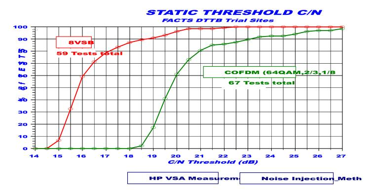
The cumulative distribution below shows the extending towards the higher threshold C/N for "dynamic" conditions. The comparison between COFDM and 8VSB may not be completely accurate as the sample is small, but it does indicates the trend of the stretching of the range of Threshold C/N to be allowed for in planning.
