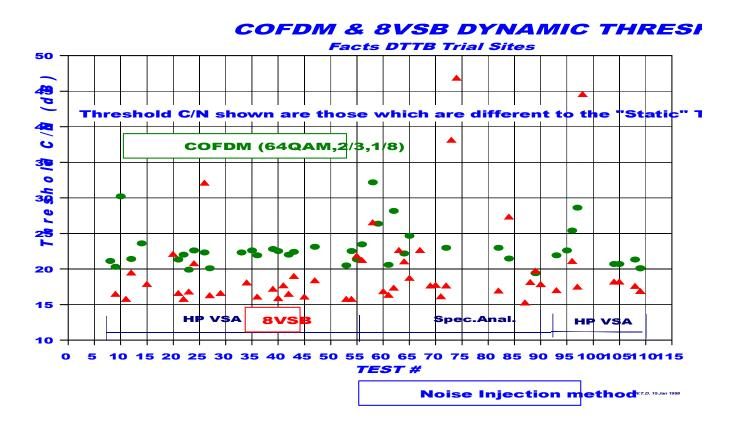
The dynamic threshold condition was defined as any random or periodic affect causing a variation from the static threshold. The conditions which caused this variation from the static threshold were more than obvious to the observer on all the occasions in the field trial. The PAL receiver was always observed to classify the character.
