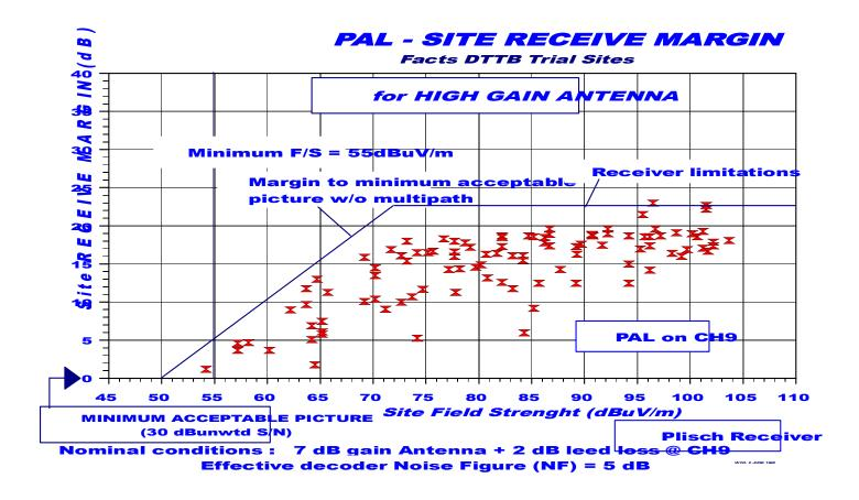
The minimum acceptable picture is defined hear as picture with a video S/N of 30 dBunwtd.
