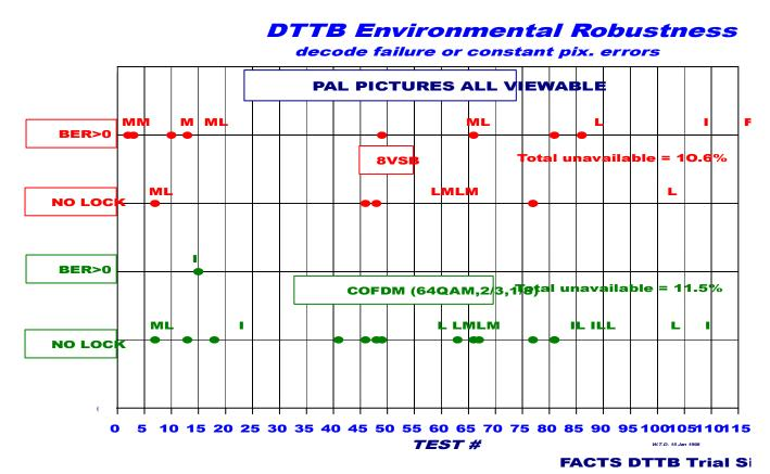
L - LOW LEVEL(PAL <=50dBuV/m) M - MULTIPATH I - IMPULSE NOISE
