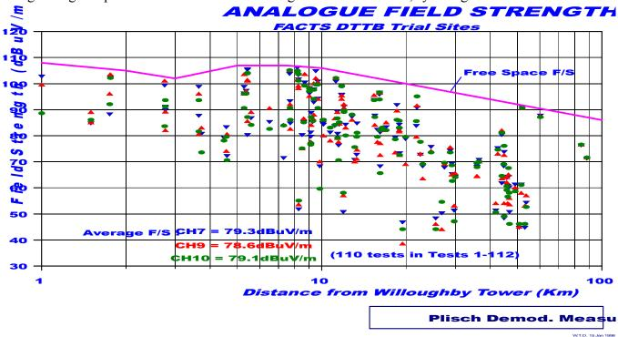
The measured Video S/N shows the relationship that F/S has to the quality of the PAL signal and allows in this Field Trial to compare to the DTTB transmissions to ascertain coverage comparisons.
