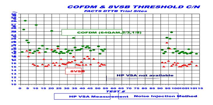
As above but using the System Attenuator method to generate the Threshold C/N. the figure shows a significant difference from that of the Noise Injection method. The system Attenuator method is closer to real environment and clearly with its higher spread of threshold C/N is the harder test.
