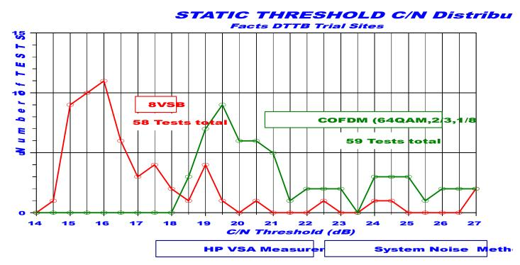
Statistics: 8VSB: Median = 16 dB Average = 17.3 dB Minimum = 14.7 dB COFDM: Median = 19.6 dB Average = 20.7 dB Minimum = 18.2 dB
